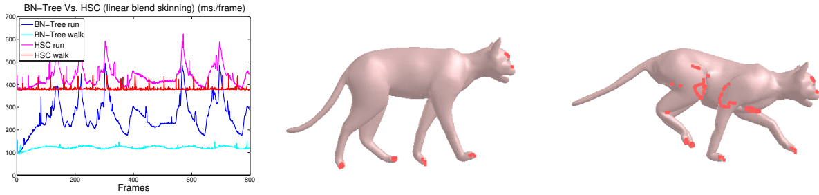
Figure 3: On the left, performance comparison between BN-Tree and [VMT94] for a cat animated with linear blend skinning, in two different situations: walking (middle) with sparse self-collisions, and running (right) with many self-collisions.
