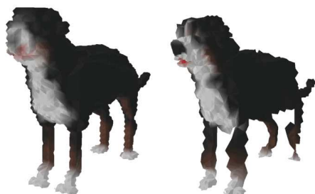
Figure 6: The non data-driven (left) and the data-driven (right) intermediate meshes for the dog model at 3 bps
