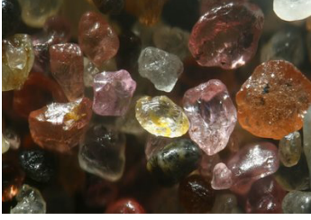
Figure 2: In a microscopic view of sand grains, we can see the irregular shapes that conform a granular medium.
